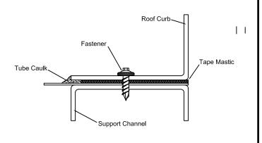
8) Apply tube caulk to full perimeter of flange edge.
