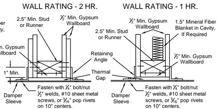
**2. Damper Sleeves and Breakaway Connections:**
