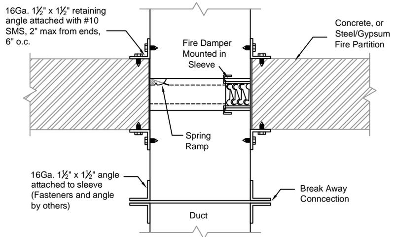
The multi-blade type fire damper installation is the same as the curtain blade type fire damper shown. This instruction sheet has been reviewed and accepted by Underwriters Laboratories,
