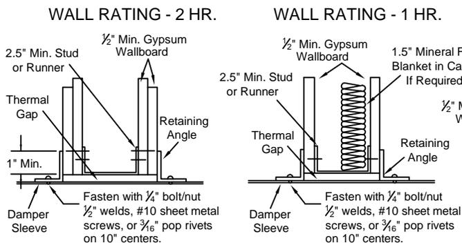
**Fig. 2: Wood Stud/Gypsum Wall Design**
